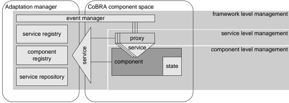
Figure 5: CoBRA architecture
