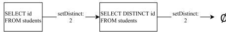
Fig. 1: Two subsequent applications of an edit with cost 2 called setDistinct on a query.
